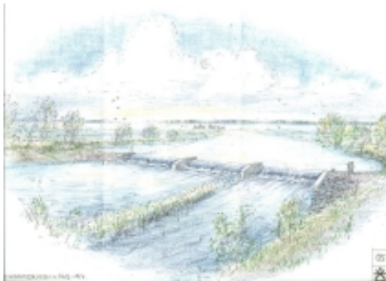
Outline of the planned dam with three tilting gates. In the new proposal the dam has two gates instead.
